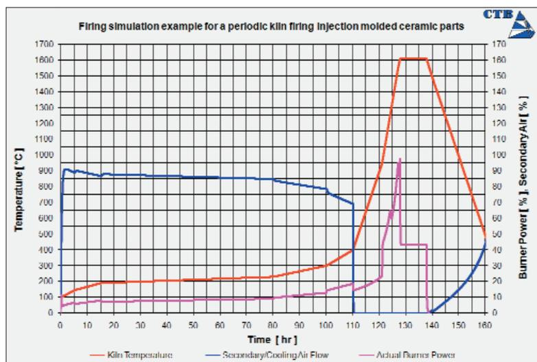
Fig. 1 For a defined optimum firing curve (red line), the energy requirement of the burner is well below 10 % in the first 80 hours of the firing cycle. To enable control of the process, however, it has to be operated at this output level. The volume of secondary air shown here (blue line) is necessary for temperature uniformity as well as for the firing atmosphere. Burners that do not cover the lower control range are not suitable for this model process
