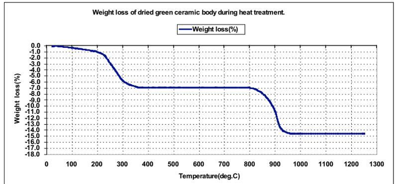
Fig. 2 Weight loss of dried green body during heat treatment
