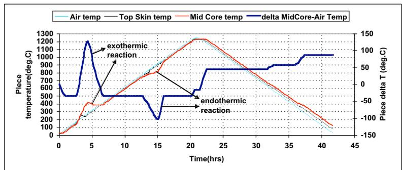
Fig. 3 Temperature distribution in green body during heat treatment
