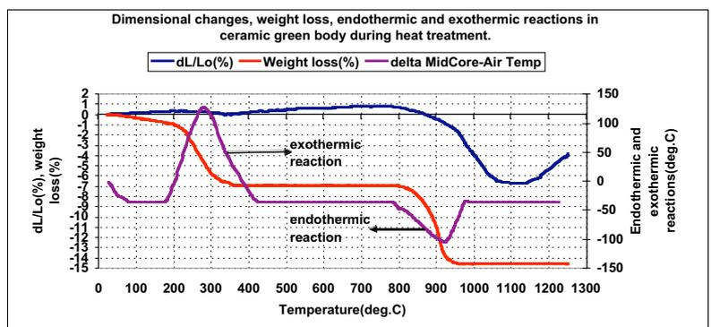
Fig. 4 Dimensional changes, weight loss, endothermic and exothermic reactions in green body during heat treatment
