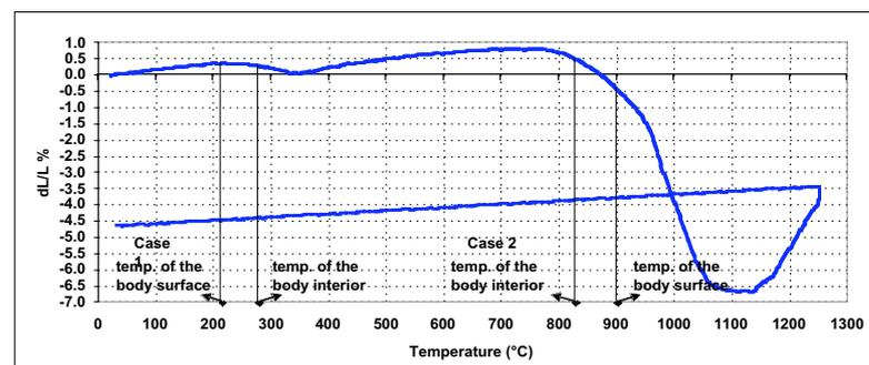
Fig. 1 Dimensional changes of green body during heat treatment
