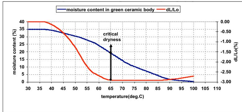
Fig. 5 Weight loss and  $dL/L_0$  in wet green ceramic body during drying
